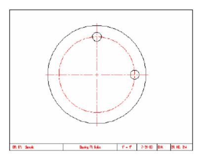
3. You are going to use the **Polar Array** command on this assignment as you did on the previous assignment. In this **assignment pay** close **attention** to the **fill angle option settings** (**number** of **items 8** and angle to **fill 135 degrees**). Select the top ½" **diameter circle** for the object to array.
