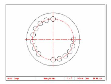
8. Array this center line using the polar array option 2 items and a fill angle of 135.
