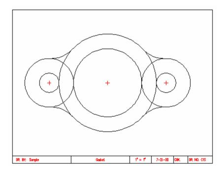
2. Select the Trim command and select the four fillet radius lines as the cutting edges.
