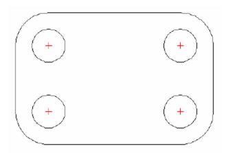
3. Change back to the **center line** layer. Use the **distance tool with** the **midpoint snap** to **locate** the **center** of the drawing **as illustrated** then **move** the **cross hair** up **2**" for the **second blip** that **marks** the **middle** of the **drawing vertically**.
