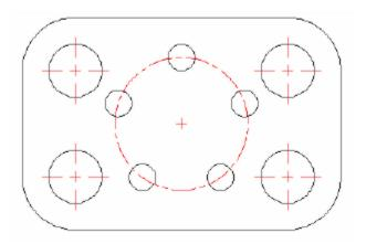
8. **Complete all** of the **linear dimensions**, **leader dimensions**, and the **diameter** and **radius dimensions** as illustrated below:
