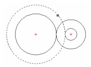
5. Position the pick box onto the larger circle to the right (1 <sup>1</sup>/<sub>4</sub>" radius circle).
