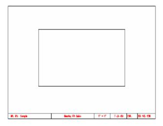
3. Select the **Fillet command from** the Home Tab Ribbon Bar and set the **radius** for the **fillet** to **1**". **Position** the **pick** box **over** the on the **top horizontal line**.
