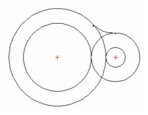
7. Repeat the fillet command on the bottom half of the drawing.
