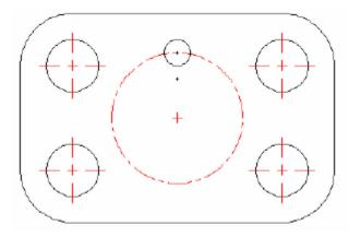
7. Complete the array command of the other <sup>1</sup>/<sub>2</sub>" diameter circles around the center line circle.
