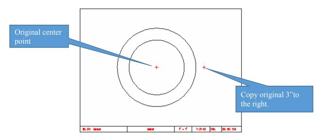
4. Change back to the object layer and draw the two circles using the copied center point mark. Draw the larger circle using the circle command center radius (1 <sup>1</sup>/<sub>4</sub>" radius). Draw the inner circle using the circle command center diameter (1" diameter).
