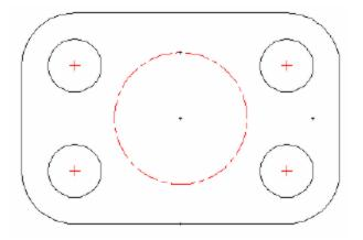
5. Continue drawing the center lines on the drawing. They will help you locate the center points for the <sup>1</sup>/<sub>2</sub>" diameter evenly spaced holes around the center circle.
