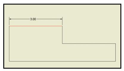
(To make the dimension number larger, click Hide Dimension Value and enter in the measurement of the line, zoom in to see the number, and highlight it using your mouse. Once you highlighted, hold Ctrl+Shift and press > until it is large enough to read without zooming in.)
