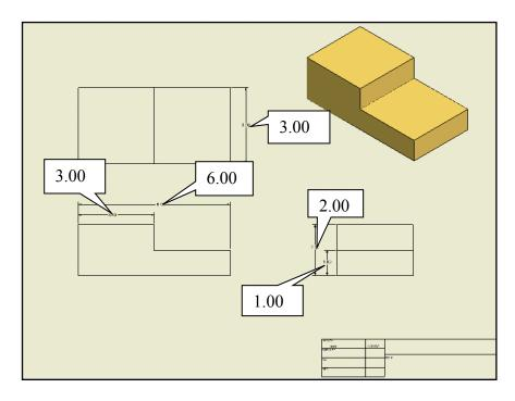
5. This activity did not include holes or circles, but later you will need to know how to dimension those. When dimensioning a circle, you must include center lines, the radius or diameter dimension, and the location of the center. The center line tools are found below for later reference.
